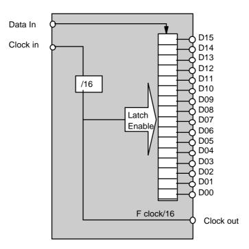
Fig.1 : Generic functional diagram of a commercial demultiplexer
