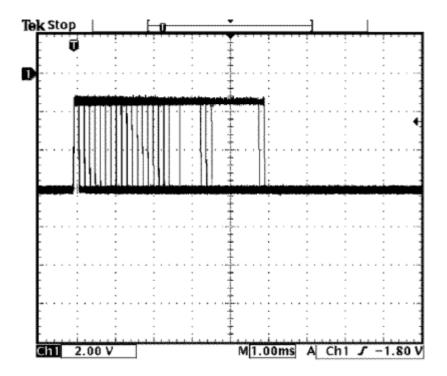
Fig.5: Random time required to get lock, for 100 successive acquisitions.
