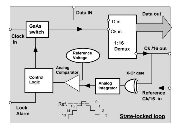
Fig 2. Block diagram of the loop
