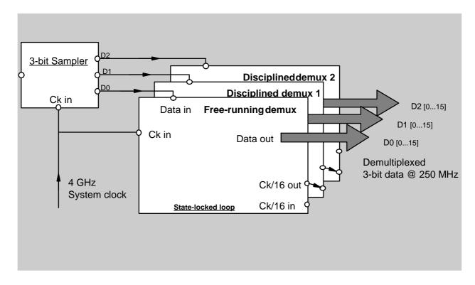
Fig 3. Cascading of loops for multibit operation
