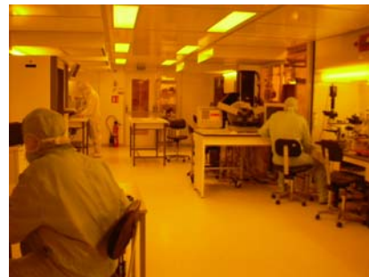
Class 100 Clean Room at IRAM for the fabrication of SIS junctions and HEBs
