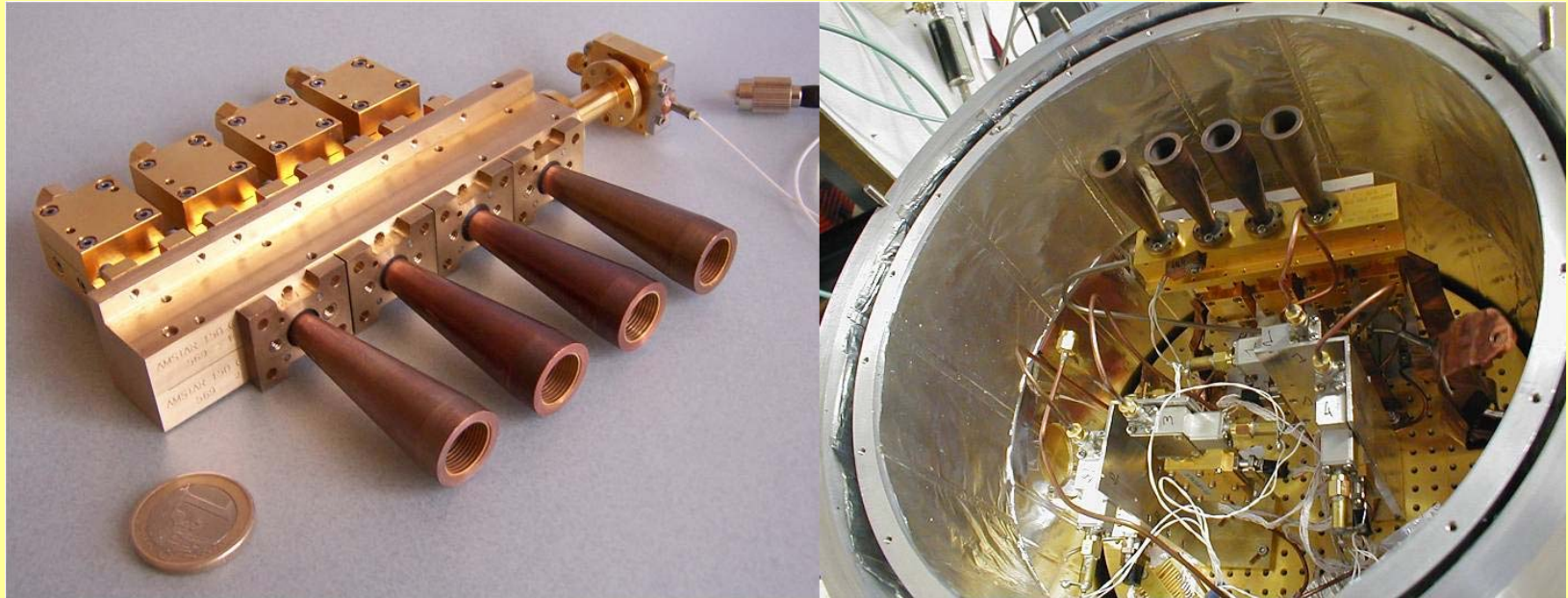
Figure 1: left: Four pixel-RF module, comprising corrugated horns (front), LO coupler (middle), DSB mixer blocks (left rear) and photomixer (rear right). Right: 4-pixel module inserted in the demonstration cryostat
