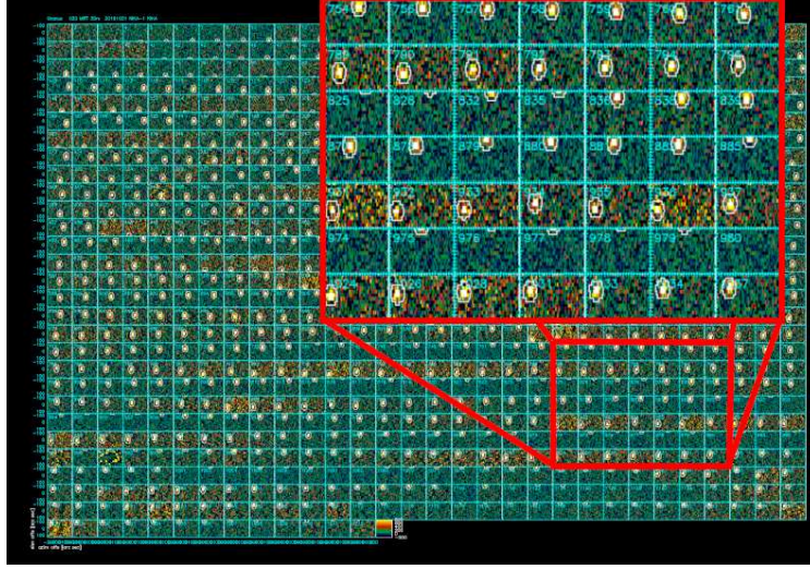
Figure 3.4: Array-1 scan maps of each individual KID, during the Uranus observation already shown in Figs. 3.2 and 3.3. The ellipse defining the area covered by the source is depicted. Those records “seeing” the source (ellipse) are not used to compute baselines.
