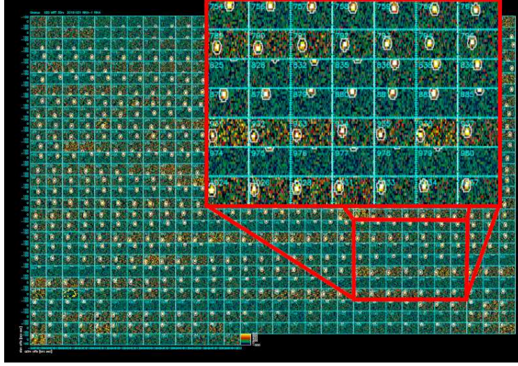
Figure 3.5: Array-1 scan maps of each individual KID, during the Uranus observation already shown in Figs. 3.3 and 3.4. The ellipse defining the area covered by the source is depicted. Those KIDs “seeing” the source (ellipse) at the given record along the timeline are not used to compute baselines for that record.
