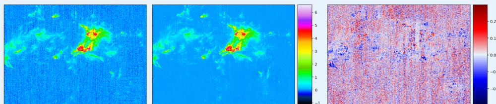
Example of noisy and denoised channel and the residues for <sup>13</sup>CO (1-0).
